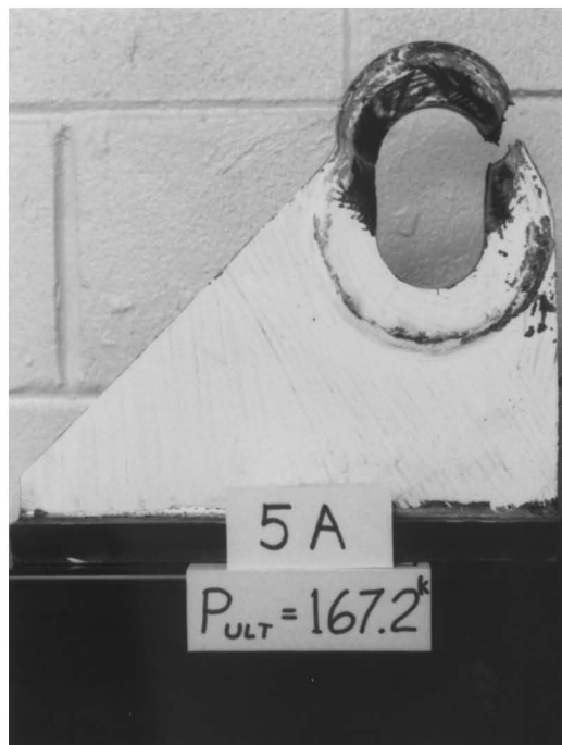
Fig. A81 - Specimen 5-A After Failure
