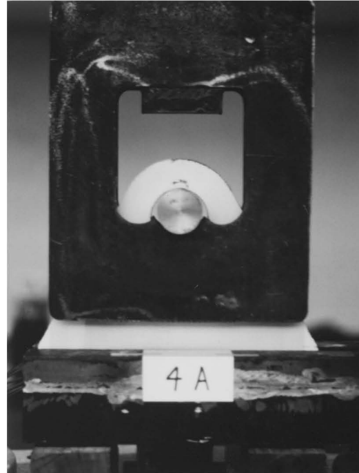
Fig. A73 - Specimen 4-A at 45.0 kips
