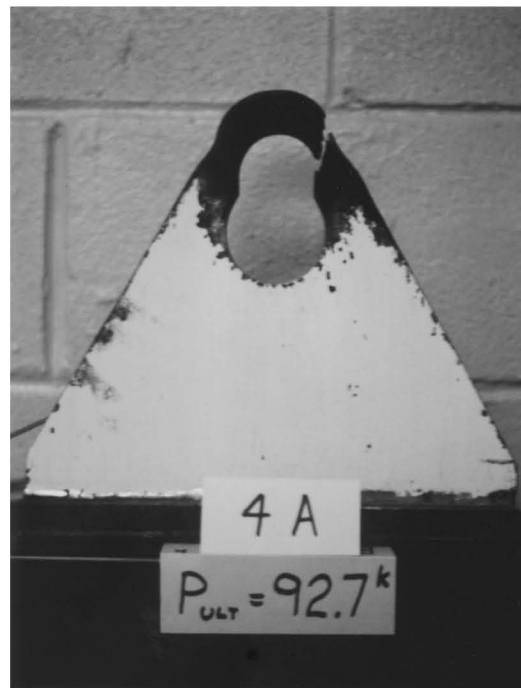
Fig. A75 - Specimen 4-A After Failure
