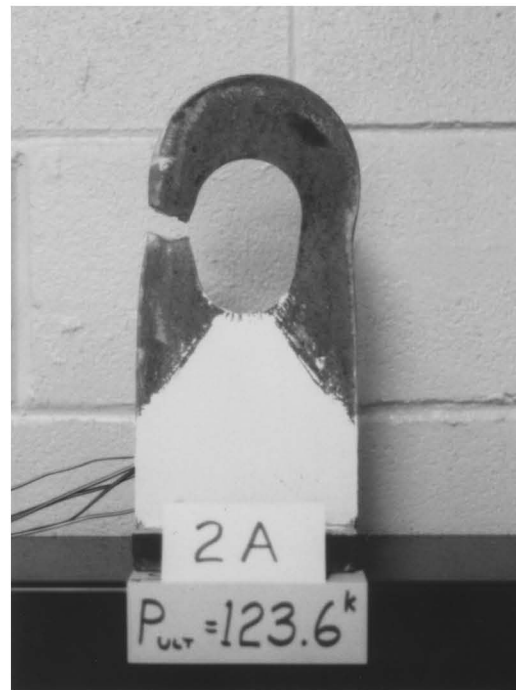
Fig. A40 - Specimen 2-A After Failure
