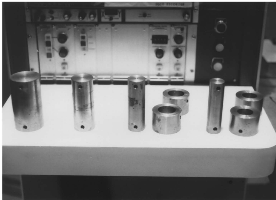
Fig. 28 - Load Pins After Tests
