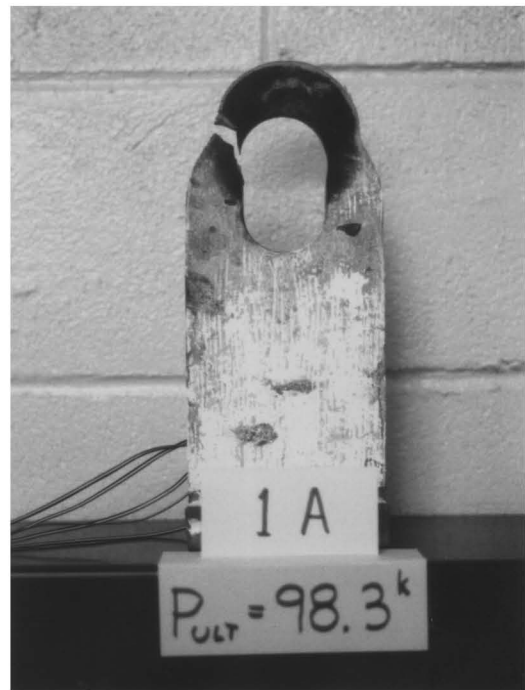
Fig. A5 - Specimen 1-A After Failure
